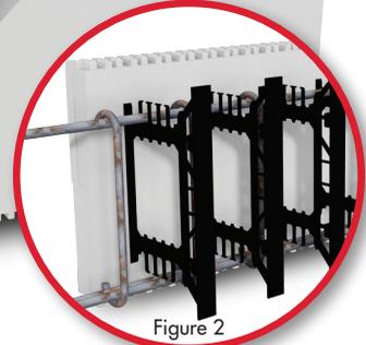
**FIGURE 2.** Rebar stirrups as required by local building codes, tying the horizontal rebar together above window and door lintels. The horizontal rebar runs continuously as required by building codes and additional reinforcement as required by engineer of record or local codes.
