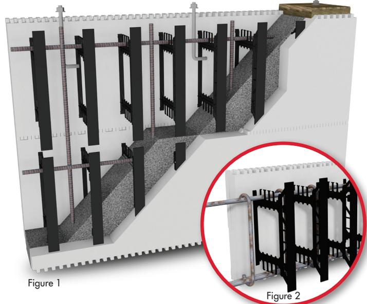
**FIGURE 1.** BuildBlock ICF wall section cutaway shows horizontal and vertical steel placement, alternating rebar placement to hold vertical rebar, J-bolts mounted in the concrete and a wooden top plate.
