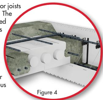
**FIGURE 4.** Integrate BuildDeck or other ICF flooring system directly into the ICF wall by cutting blocks at the correct height and joining the floor and wall systems during a continuous pour.
