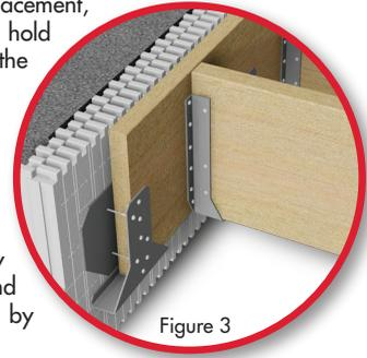
**FIGURE 3.** Attachment of standard floor joists to an ICF using traditional lumber. The Simpson Strong-Tie ICFVL is embedded into the poured concrete and provides mounting for wood or steel ledgers.
